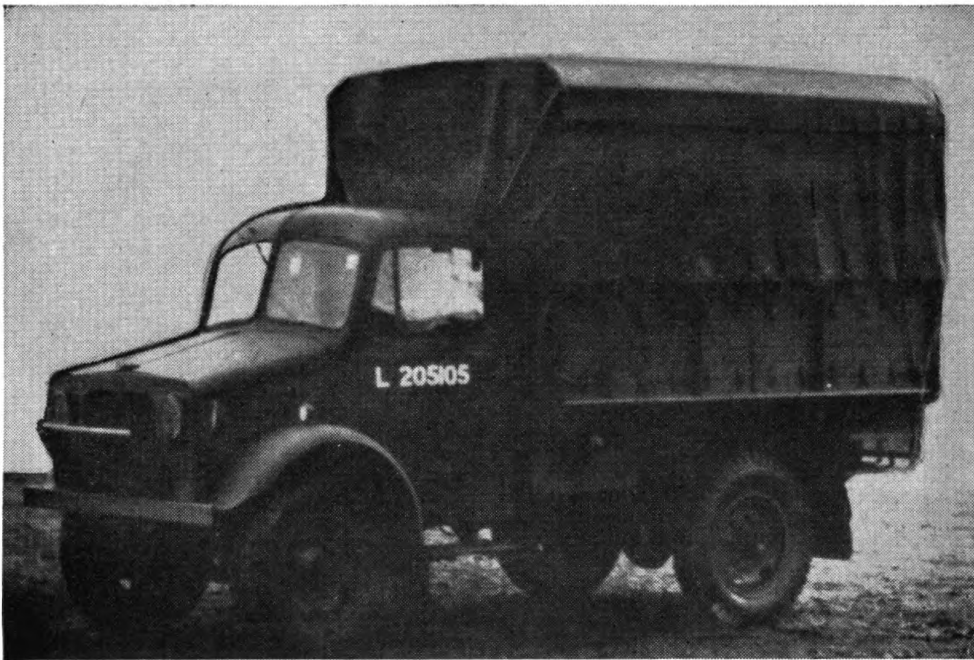
FIGURE 103.—30-cwt general-service lorry (Bedford OX).
